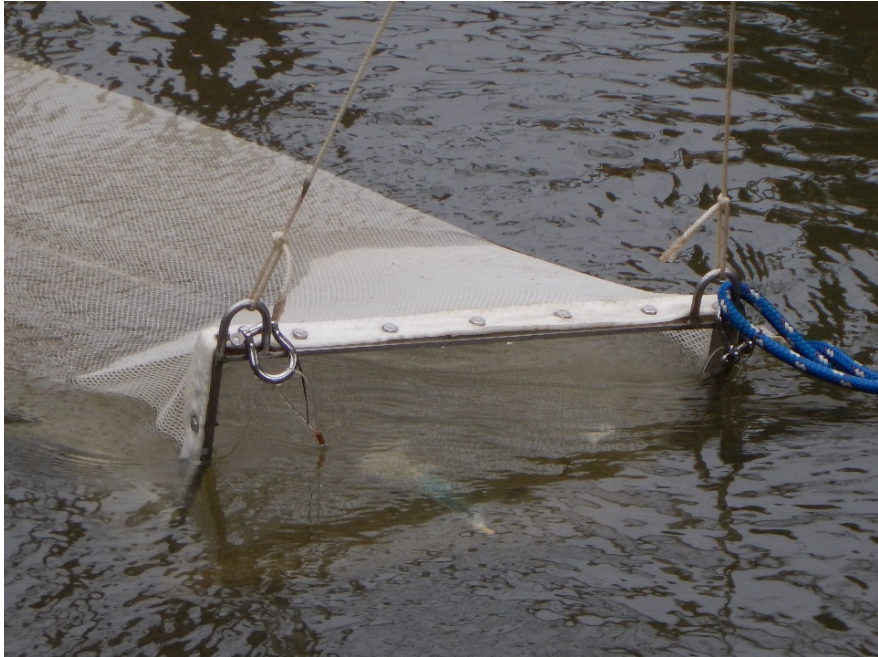
Figure 10. Rectangular Trawl with flow meter attached at San Mateo Creek
